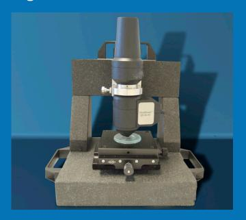
The DS-95 Compact Granite Stage provides the possibility of investigating nearly all samples by SPM.
