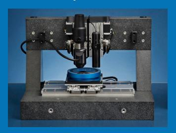
Since the DS-95 Navigator 220TM is released the statement "You will never again find this spot with your AFM" is no longer true. The DS-95 Navigator 220TM enables to investigate one and the same area again even after removing the sample from the AFM. Based on reference structures the system finds the area of interest with a precision better then 250nm.
