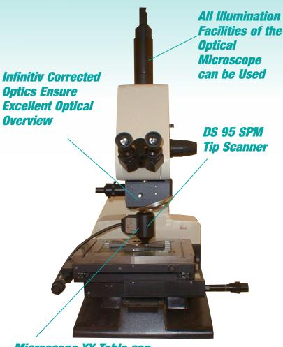
*Microscope XY Table can be used to Navigate on the Sample.*
